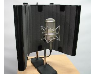
Tight. Very dry sound with attenuated treble response
